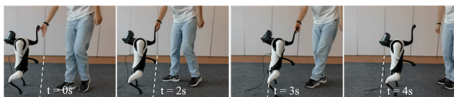
Fig. 9: A human walks hand-in-hand with the standing quadruped robot and drags its front leg to change its position.
