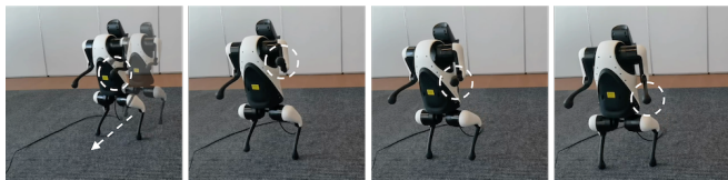
Fig. 8: Using LLM to generate motions for walking forward a few steps and then waving the left hand up and down.
