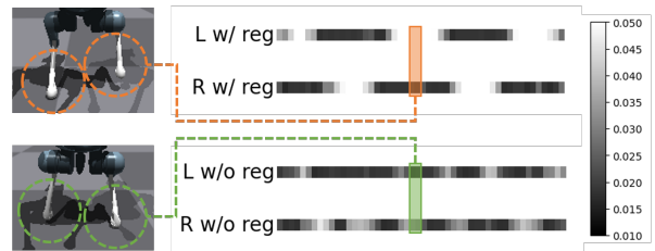
Fig. 10: The feet heights recorded along the execution of different policies in simulation. Darker colors indicate the lower heights. Top: The left and right foot heights of the policy trained with our feet regularization reward terms, which demonstrates nice feet clearance. Bottom: A policy trained without these regularization terms tends to slip on the ground and can hardly be transferred to the real robot.
